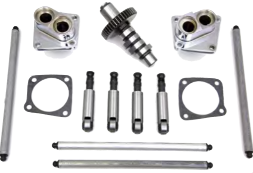
Performance Cam Kit Sifton performance cam kit includes cam, solid lifters, pushrods and chrome lifter bases. Cam lift is .412 for 1970- Early 1977 Shovelhead models.
